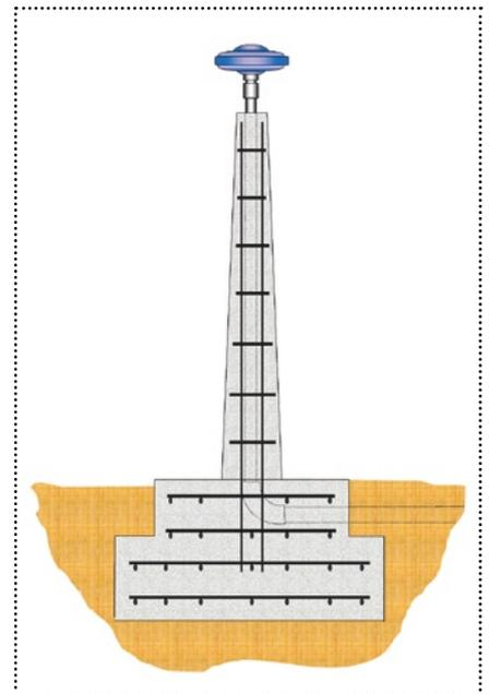
One of many similar variations. this seeks to provide a heavy-stable base for a pillar. Reinforced concrete provides mass, with a broad base. Some have experimented with low, squat pyramids, but those can present a multi-path hazard; the pillar
