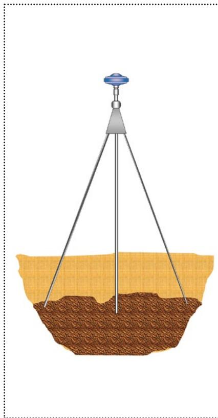
This can be used when the depth to bed-rock or other stable surface is less than 10 feet. The stability of a tripod (though most constructed have 4 angled legs plus one vertical under the antenna) is paired with narrow members (to reduce multipath hazards). This is very popular with the scientific community, okay by both Unavco and NGS standards.
