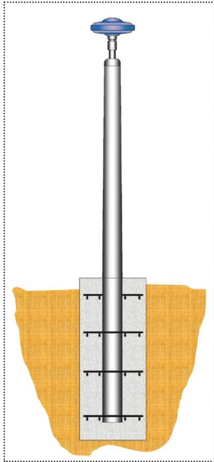
There are several variations on this theme: one involves pounding a pole or “I-beam” down to refusal (or as far as one can afford), another style sets a pole (like a spun-aluminum light standard) down into an augured hole filled with concrete. On some pole type mounts 2-axis tilt-sensors have been added to monitor stability.
