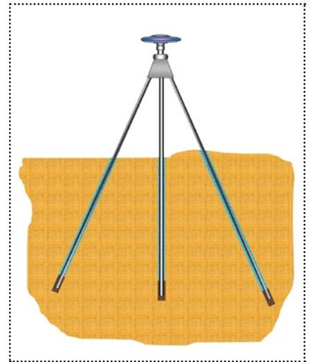
Another tripod, “quad-pod”, or “quint-pod” style monument, this one is used where the soil and sub-surface conditions may be less stable. The legs may be drilled up to 40 feet and only cemented into place at the very bottom; the balance of the hole around each leg is filled with an insulating material that will not place drag on the legs in the event of shallow strata shifting or sub-surface expansion-contraction.
