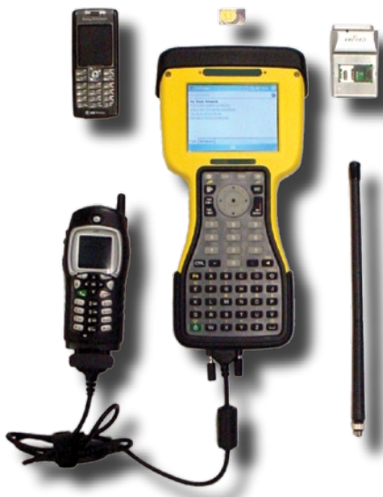
Figure 2 Rover components often accommodate multiple communications options. This data collector offers (clockwise from upper right): a slot for the compact-style cell card, connections for a rover radio and antenna, serial and USB ports for connection to cell via cable, connection to cellular via Bluetooth. The unit itself (center) has built-in WiFi capability. Also pictured (at top) is the SIM card that fits into cellular devices containing the user account information.
