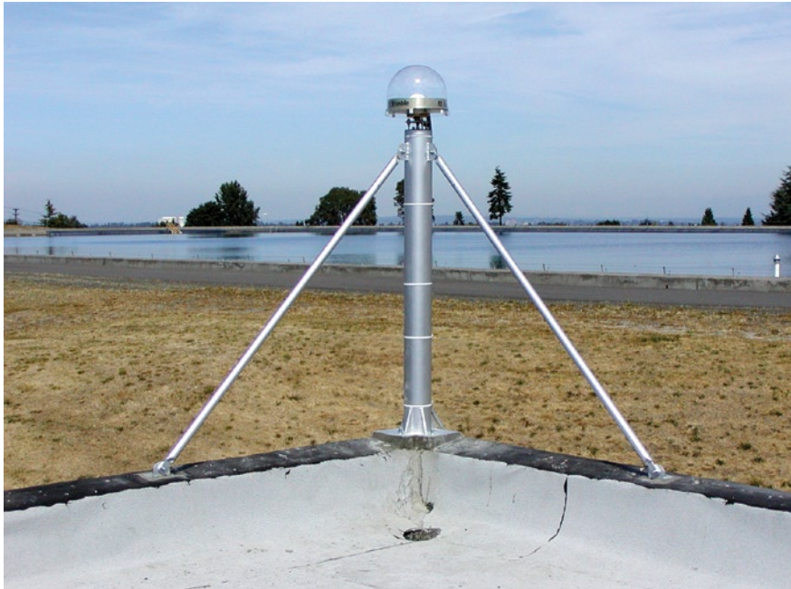
Reference Station at West Seattle Reservoir: originally established for plate tectonic studies and resources mapping, it was added to the state network with no modifications needed.
