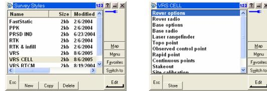
· Under [Rover options] the “survey type” field should be [RTK]; “Broadcast format” should be [VRS (CMR)]; the other fields should stay the same.
