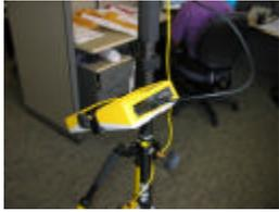
8. Connect Trimble TSCe data controller data cable to the center LEMO port on the TSCe data collector. Connect the other end of the TSCe data controller data cable to the #1 port (with data collector symbol) on the Trimble 5700 GPS receiver.
