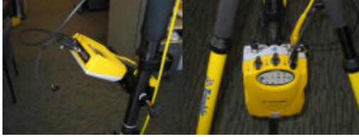
9. If you want you can tidy up the cables by strapping the cables to the bipod rod with the Velcro straps.
