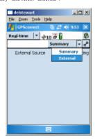
When connected to 4 or more satellites, radio icon will switch from blinking to solid, indicating connection to VRS/Base Station and status below will show duration connected, data received, etc. -If VRS link fails, verify internet connection, IP address settings, Port number and user name info. 15. Tap the ArcPad Icon above the wrench to return to map screen where you can collect data.
