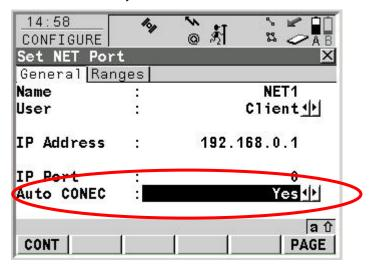
?? A second NET port needs to be configured with the **User** prompt set to **Server** (this Net port operates than as a TCP/IP Server)in order for the GPS Spider software to connect to the sensor.
