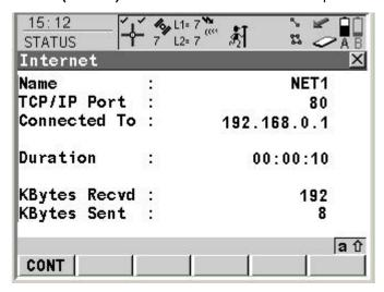
The **STATUS Internet** panel shows the **Duration** of the connection for the individual Net port from the time the connection is established till the moment the Net port is disconnected from the Server. Also shown is how much data is sent or received in that time period.
