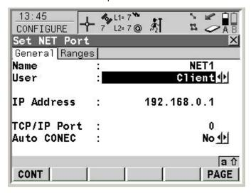
As already mentioned, when using GPRS to access the Internet it is only possible for the sensor to act as a TCP/IP Client due to the dynamic IP address of the sensor. Therefore set the **User** prompt to **Client** and enter the **IP Address** of the Server (Broadcaster) to where the Net port should connect.
