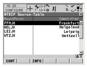
Move the focus to the required Mountpoint and press F1(CONT) to copy the Mountpoint name to the **Mountpnt** prompt in the **NTRIP** page of the **CONFIGURE Additional Rover Options** panel.
