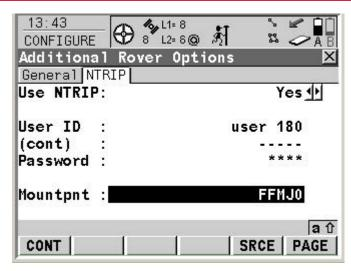
In order to access and receive RTK data from the NTRIP Caster a **User Id** and **Password** needs to be entered. If necessary, contact your NTRIP administrator to obtain a User ID and password.
