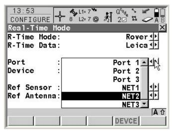
Note, these new ports should be treated in the same way as the "normal physical" ports (Port1, Port2 and Port3) – this means that only one port is allowed to be used with one Interface.
