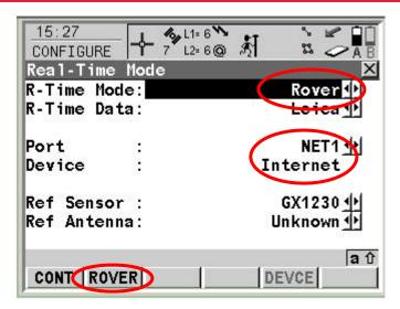
To configure the NTRIP specific parameters press **F2(ROVER)** to access the **CONFIGURE Additional Rover Options** panel and select the **NTRIP** page.
