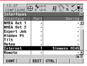
Access the **CONFIGURE Interfaces** panel, place the focus on the Internet Interface and press the **F3(EDIT)** button to access the **CONFIGURE Internet Interface** panel. The Interface specific parameters can now be configured.
