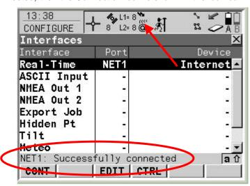
RTK data would now be received from the Server (e.g. the NTRIP Caster) and the RTK arrow would flash to indicate RTK data being received.
