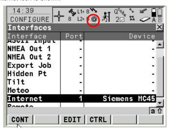
The sensor is now online to the Internet, but because GPRS is being used, no charges are yet made since no data transfer from the Internet has yet taken place.
