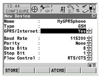
Select **Yes** at the new **GPRS/Internet** prompt. This informs the sensor that this device is GPRS capable and allows AT commands to be entered which will steer the GPRS functionality of the device. The
