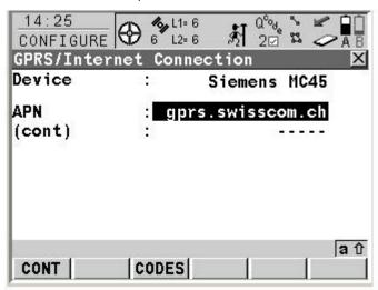
The **APN** can be thought of as the "home page" of the telecom provider using GPRS for accessing the Internet. Contact your telecom provider to get the correct APN name. The following web site gives an overview of the different parameters (APN, User ID, password) for different telecom providers <a href="http://www.access-sys-eu.com/GPRS\_Settings.95.0.html">http://www.access-sys-eu.com/GPRS\_Settings.95.0.html</a>. Note, the accuracy of this information cannot be guaranteed.
